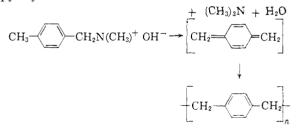
*p*-Xylylene, produced by fast flow pyrolysis of *p*-xylene in gas phase, can be isolated in solution by instantaneous condensation of the pyrolyzate in a cold solvent. Hence, it appeared probable to us that degradation of the appropriate quaternary hydroxide might be a convenient method for isolating a variety of xylylenes, if the procedure could be modified to enable removal of the transient intermediates from the reaction flask as fast as
